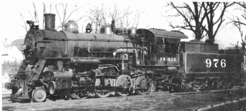
wheels. The first number indicated the number of wheels in the leading truck, the second number listed the driving wheels, and the third number was for the wheels on the trailing axle.
