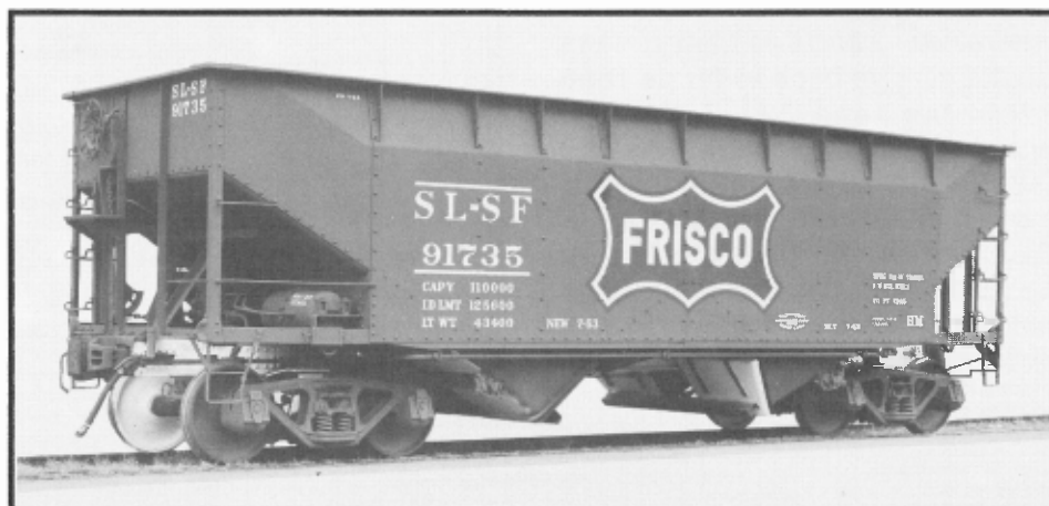
Frisco Twin Bay hopper #91735, series 91600-92399. Pullman Car Co. Chicago, IL July 10, 1953 Pullman photo
