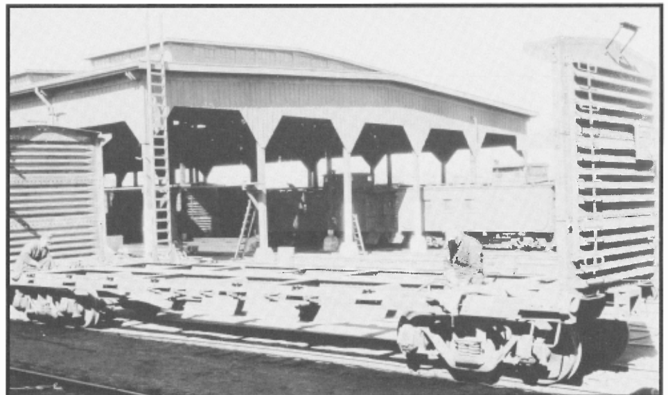
Frisco 127000-130519 series box car stripped to steel ends, frame, and trucks, Springfield, MO, February 23, 1935.
