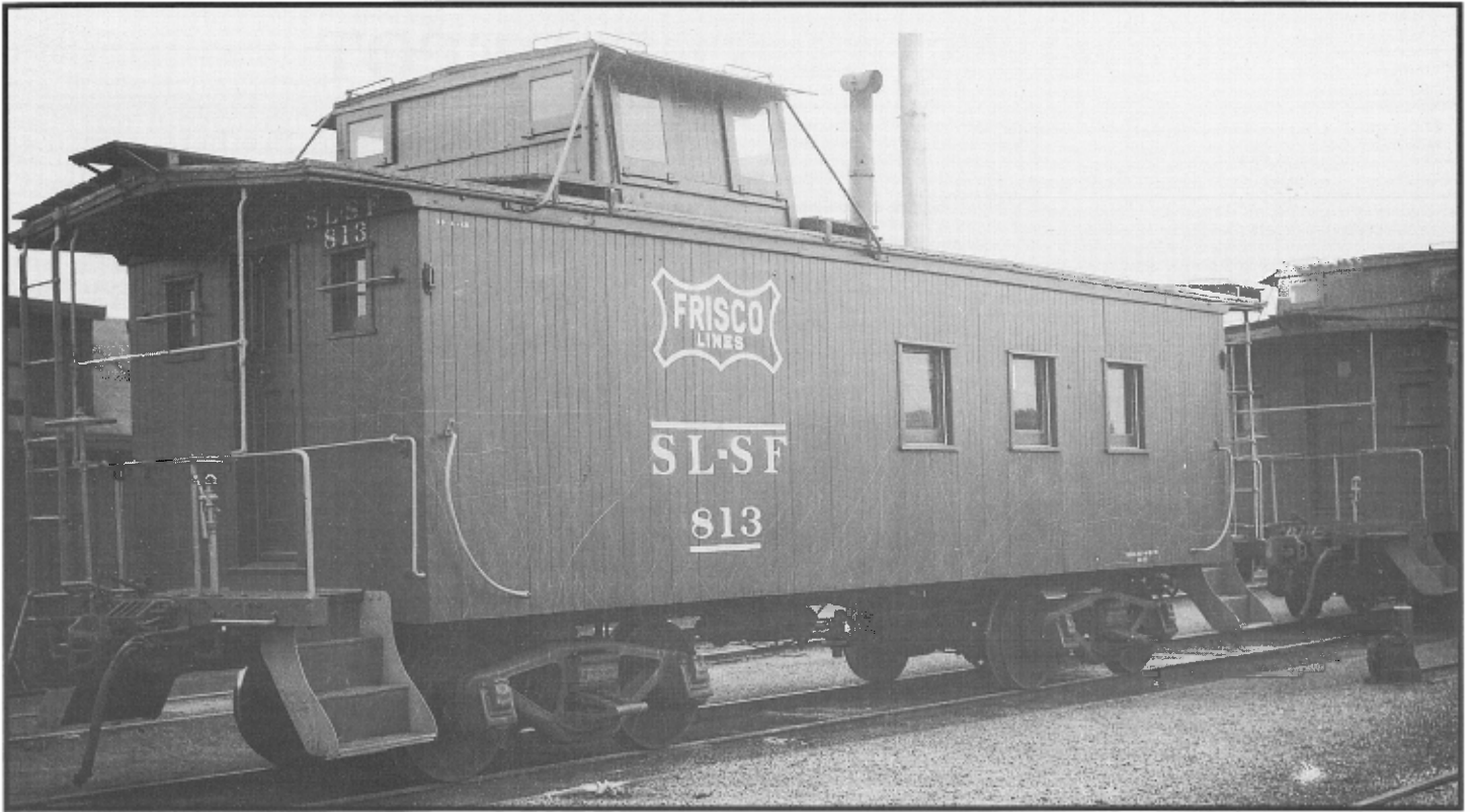
SL-SF 813, in service at Pittsburg, KS, May 30, 1948. Items and modifications to note: 1) Addition of end windows. 2) New safety railing on end platform and all railings, grab irons, and step edges painted yellow (September, 1947 modifications). 3) Frisco Lines logo. A. Johnson photo
