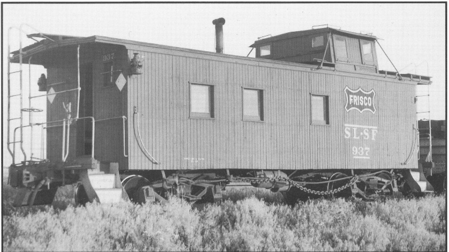
SL-SF 937, in service at Enid, OK, May 30, 1958. Items and modifications to note: 1) Spacing between second and third windows. 2) Addition of safety ladder (1938 modification made on some units) 3) Addition of 10" silver Scotchlite diamond reflectors on end of car (1953 addition). 4) Raising of platform whistle position. 5) Frisco logo.
